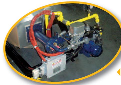
LPG/methane automatic burner with electronic ignition, for high temperatures (1350°C)
