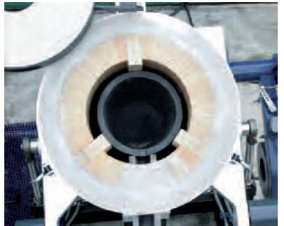
Highly refractory bricks with excellent thermal insulation. Protected with strong and metal construction
